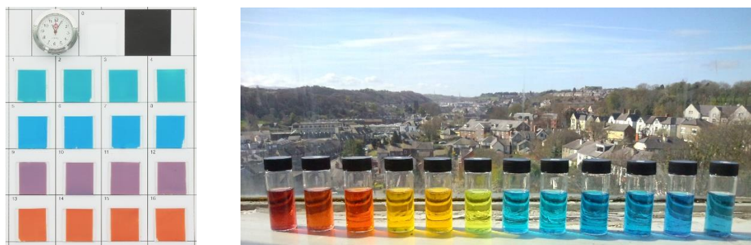
Fig.1 (Left) Sensitized photo electrodes with a range of dyes during exposure to artificial light and (right) dye solution under exposure to natural light.
