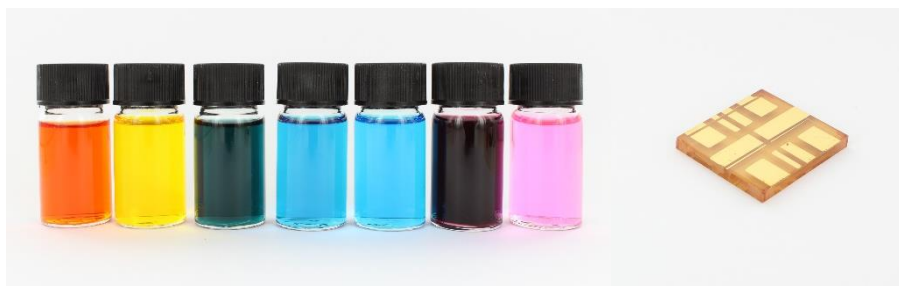
Figure 1. Different coloured dyes (left) and hole transport materials will be tested in order to maximize efficiency and stability of solid-state dye-sensitized devices (right).
