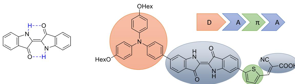
**Figure 1:** on the left-hand side the H-Chromophore is highlighted on the Indigo's structure. An example of a D-A- $\pi$ -A dye bearing Indigo as the internal acceptor is reported on the right-hand side.
