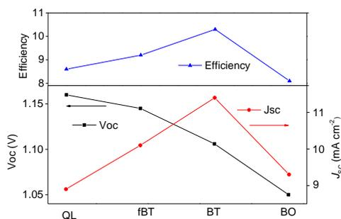
**Figure 2. Summary of the Efficiencies,  $V_{OC}$  and  $J_{SC}$  of the IDT Dyes-Based DSSCs.**
